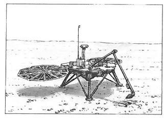
The Phoenix spacecraft reached Mars in 2008. It has a 2.4-meter (7.7-foot) robotic arm that dug into the soil to uncover a layer of ice. The arm dropped soil samples into instruments that checked for water and carbon-based chemicalsessential elements for life.
