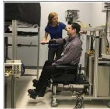
*Amanda setting up the Kinarm exoskeleton robot for an experiment.*
